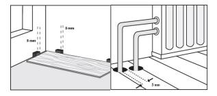
room, such as pipe penetrations, door stops, door frames and others. It is necessary to create expansion gaps between individual rooms. Expansion gaps cannot be filled with filler, electical cables and others!
