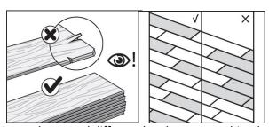
and combine different tiles, so decor pattern is not regularly repeating and eventual different batches are combined in one room. Plank format can be customized by cutting the surface with straight knife and finishing it with a sharp hook after breaking the plank-
